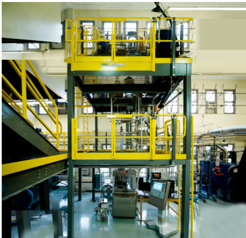
Fig. 3 The CM unit: Excipient and API hoppers and weighing units on top tier
