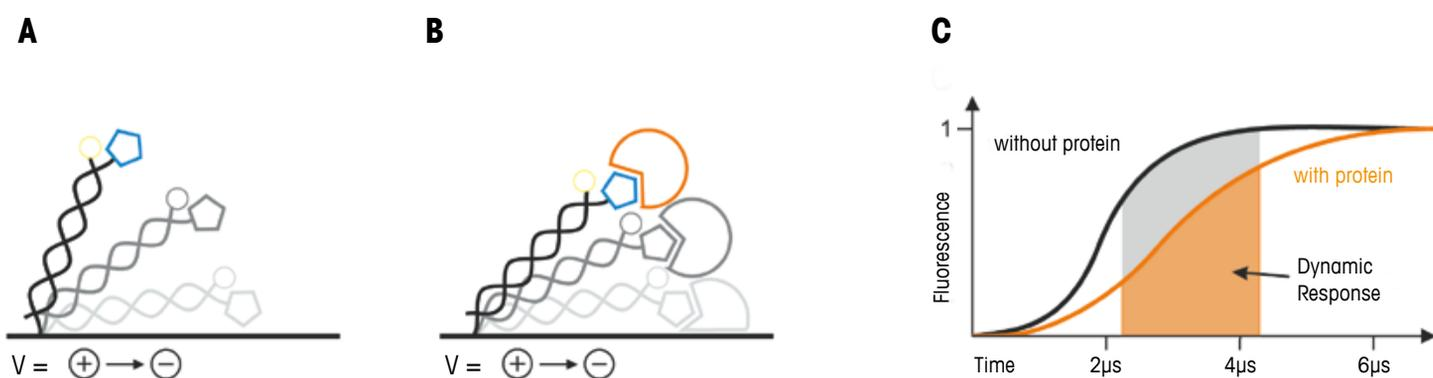
**Fig. 1** The diagram illustrates the stand-up motion of DNA (A) and DNA with a bound protein (B). The corresponding time-correlated measurement signals (black: DNA; orange: DNA with protein) are shown in C. The „dynamic response” is the area under the curve in question and a metric for switching speed.
