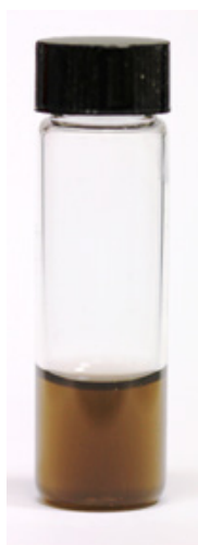
Fig. 2 Colloidal suspension of hydrogenated nanodiamonds dispersed in water (3 mg/mL)
